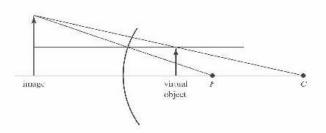
**34.68:** The derivations of Eqs. (34.6) and (34.7) are identical for convex mirrors, as long as one recalls that R and s' are negative. Consider the diagram below:
